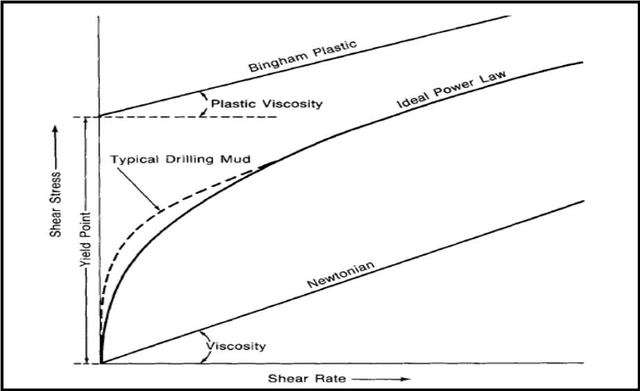
Figure 1: Ideal Consistency Curves for common flow models [1]
