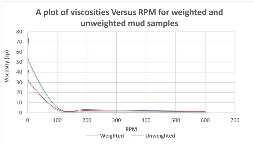
**Figure 2: Viscosities Versus RPM for weighted and unweighted mud samples**
