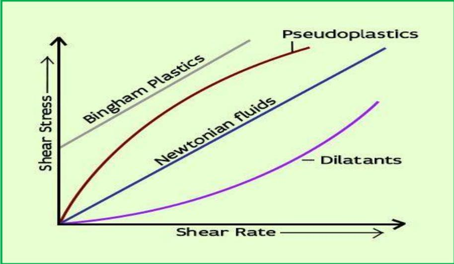
Figure 2: Comparison of shear stress, shear rate properties and yield point [2]
