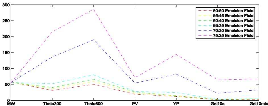
FIGURE 4. WATER-BASED EMULSION MUD IN DME AT 140 °F.
