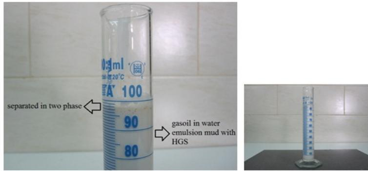
FIGURE 6. SAMPLE OF PREPARED WATER-BASED EMULSIFIED FLUID.
