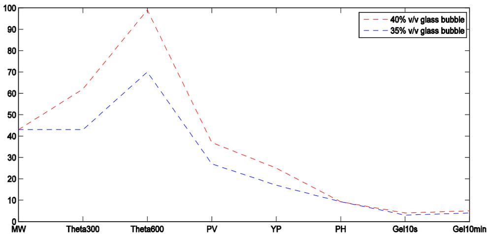
FIGURE 10. COMPARISON BETWEEN 43 PCF 70:30 WATER-BASED EMULSION FLUIDS WITH 40% V/V AND 35% V/V GLASS BUBBLE.
