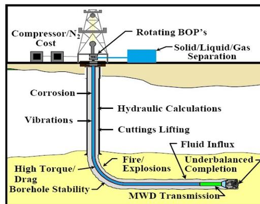
FIGURE 1. HOLE PROBLEMS WITH AERATED DRILLING FLUIDS [9].
