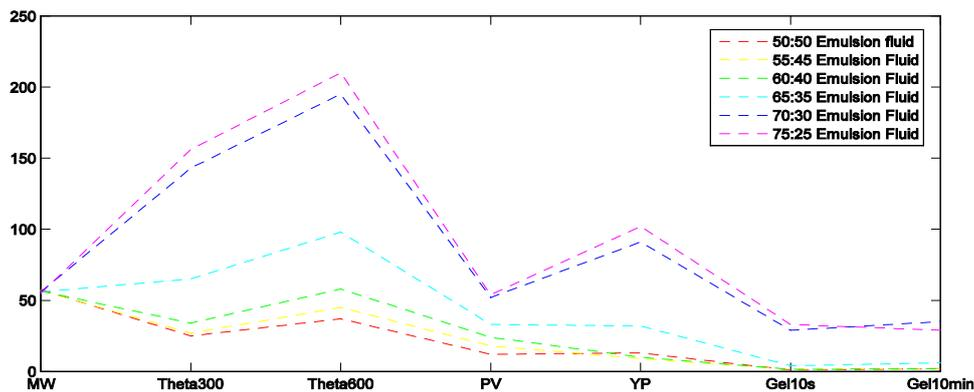
FIGURE 3. WATER-BASED EMULSION FLUID IN DME AT 77 °F.
