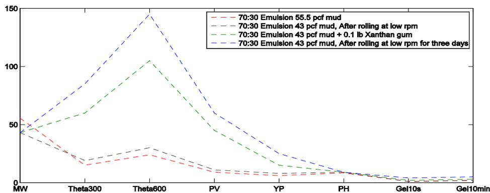
FIGURE 7. COMPARISON BETWEEN WATER-BASED EMULSION FLUIDS, AFTER 24 HRS, AFTER ROLLING OPERATION AT LOW RPM, AND AFTER 3 DAYS AT LOW RPM.
