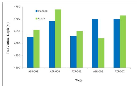
Figure 3 Actual drilled depth vs. Planned for Azar oil field wells
