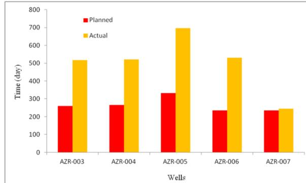
Figure 2 Actual drilling time vs. Planned for Azar oil field wells
