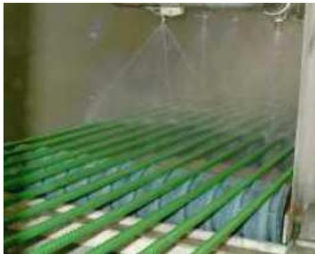
Figure 9. FBE coated rebar under water quenching
